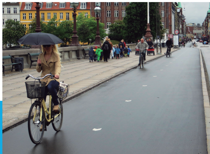
Consistency in Copenhagen, Denmark: always on the right side, always unidirectional and always physically separated from cars when car's maximum speed is above 30 kph (20mph).
