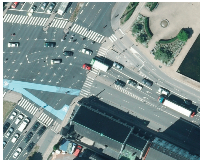
Figure 9 and 10: "Capture island" Gyldenløvesgade - Nørre Søgade, Copenhagen. The island and the signals omit the conflict between right turnings cars and ongoing cyclists (Photo: Copenhagen Municipality)
