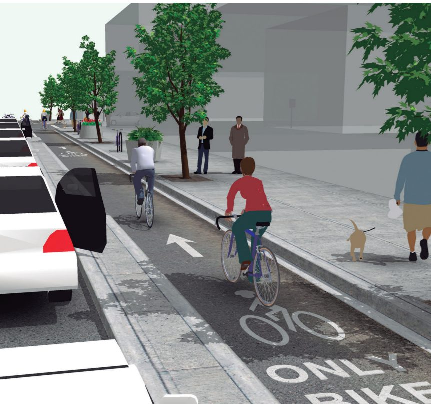
Graphic Courtesy of Alta Planning + Design One - way protected cycle track with raised curb and parking buffer. Nacto guide
