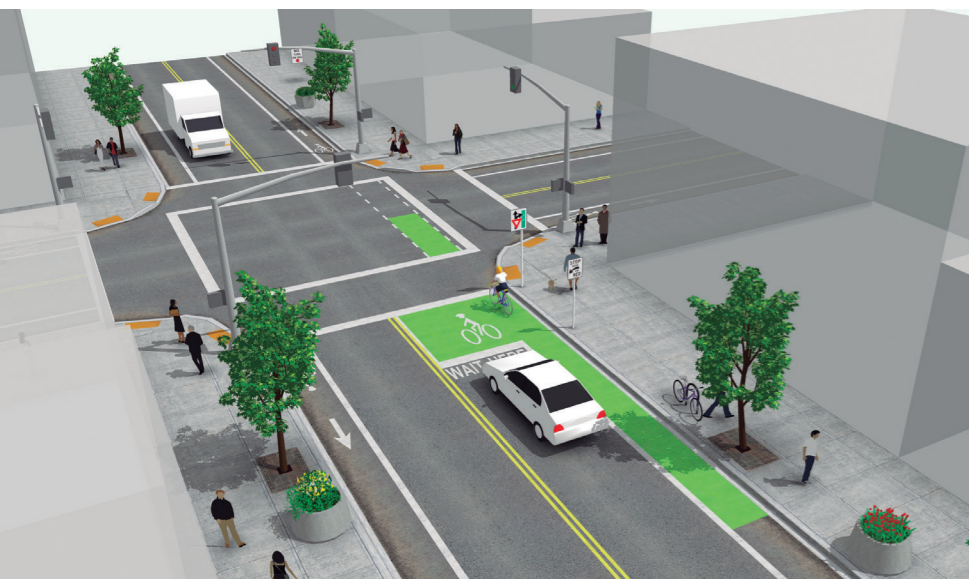
Bike box at a signalized intersection (intelligible) a bike lane approach. NACTO guide
